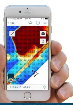
A pocket tool for managing production in the field, the SmartTrack mobile app displays real time equipment tracks from simple 4D Sensors, on a georeferenced cut-fill grid map or plan sheet, and provides your foreman or project manager with a current measure of his load counts, cycle lengths, cycle times, moving time, stopped time and location of the tracked equipment.
